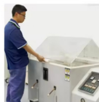
Salt-spray testing machine
